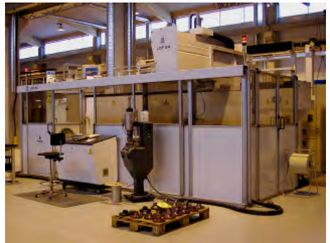
Figure 8. Industrial laser coating cell with 6 kW CO 2 laser (Kokkola LCC Oy, Finland).
