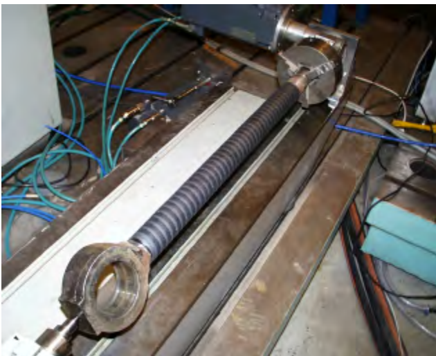
Fig. 12. Laser coated hydraulic rod. The piston was laser coated by using a high rate 6 kW HPDL laser coating process with a highly corrosion resistant coating.
