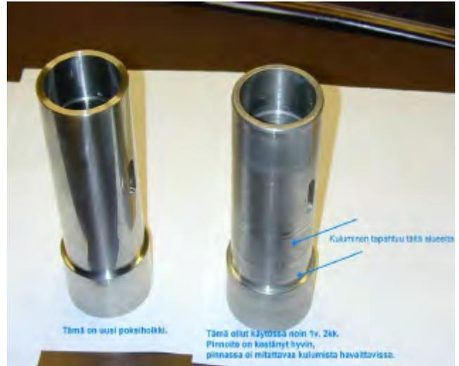
**Fig. 13.** Laser coated sleeve for highly corrosive 80% phosphous acid application. Left: unused laser coated sleeve; right: laser coated sleeve after 1 year and 2 months of operation.
