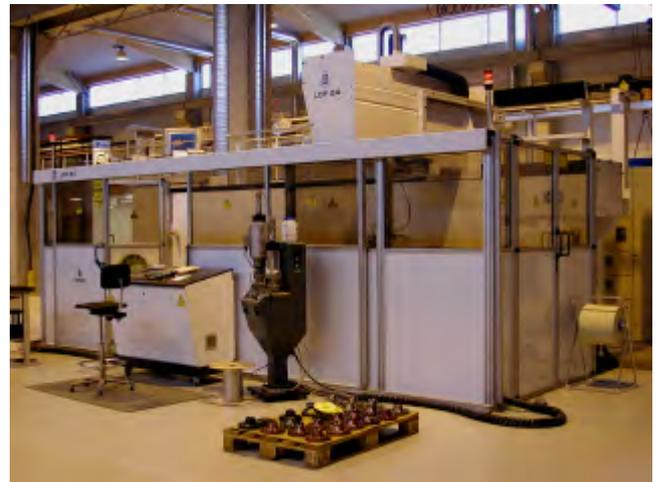
Figure 8. Industrial laser coating cell with 6 kW CO<sub>2</sub> laser (Kokkola LCC Oy, Finland).
