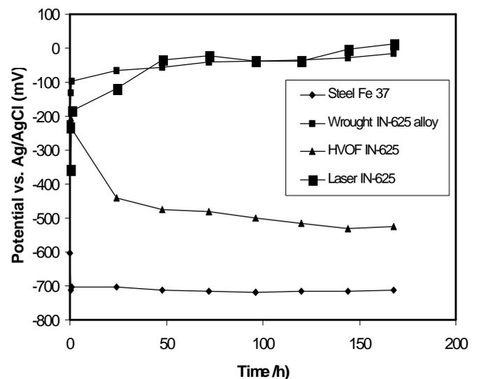
**Figure 5.** Open circuit potential vs. time for steel Fe 37, HVOF sprayed Inconel 625 coating, Inconel 625 laser coating and wrought Inconel 625 alloy.
